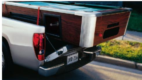
Open. Shut. Or 55°. Colorado's **TAILGATE** latches securely at 55°, aligning the tailgate lip with the top of the wheel wells to create three points of contact. Just the kind of versatility you need to secure and stabilize those awkward, oversized loads.
